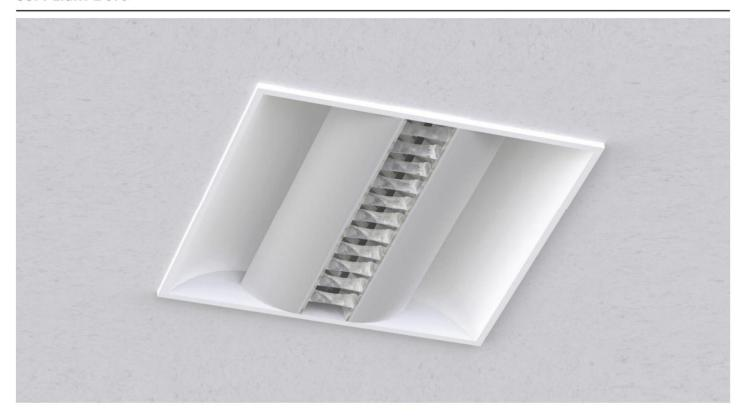
A recessed 600x600mm luminaire with special geometrical structure. The combination of the parabolic louvre and the micro-perforated reflector gives a direct-indirect light distribution, suitable for environments where diffuse and soft light is required for optimal visual comfort.
