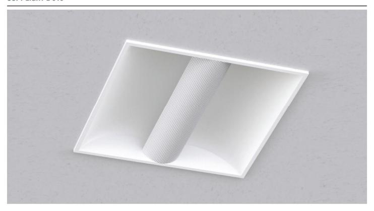
A recessed 600x600mm luminaire with special geometrical structure. The combination of the reflective recuperator and the micro-perforated lamp cover gives a direct-indirect light distribution, suitable for areas where soft, mostly indirect, illumination is required.
