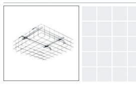
Wire-guard applications in dry environments, against shocks coming from any directions, in galvanized steel rod Ø5mm. To install it, ceiling-mounted bracket code 0213 is always necessary.
